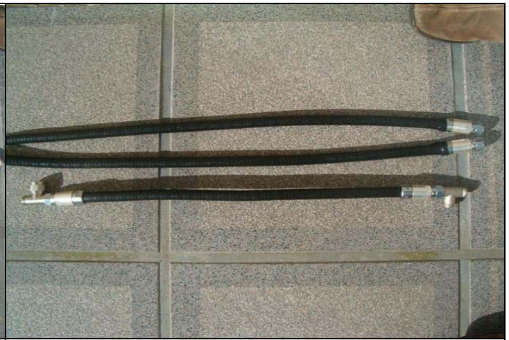
The exclusively 1/2" corrugated cables (L1 and L2)
