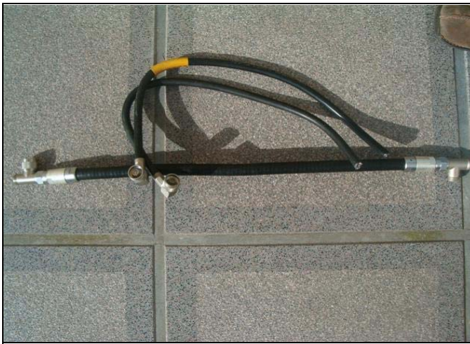
The 1/2" corrugated L1 and open ended braided cables (L2)
