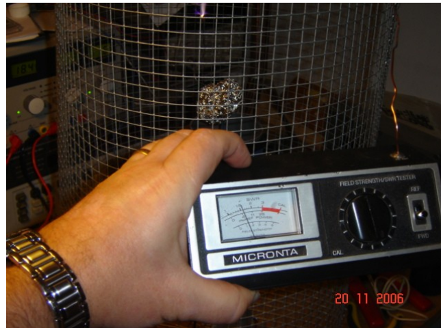
Figure 28: Using a field strength meter to check shielding effectiveness.
