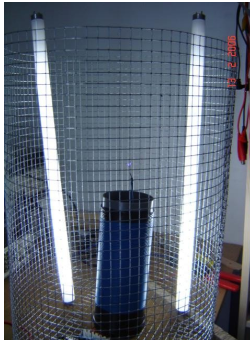
Figure 2: Picture of energised Tesla coil resonator in its "cage" with two standard fluorescent tubes.
