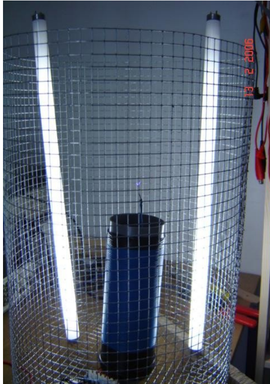
Figure 24: Coil inside of shielding cage.
